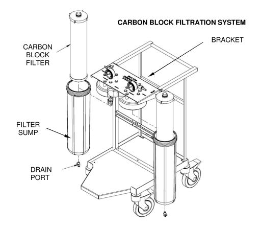
The illustration above shows the Carbon Block Filtration System installed on an M1 Cart with the filters and filter sumps removed for illustrative purposes. An RO machine is not shown.
