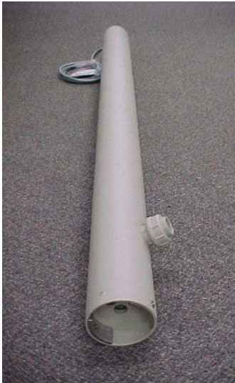
Pump with low side port
