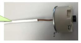
Check if the High Limit Switch has "tripped"; the blue reset button would be extending 1.7 mm past the black "set plug". The High Limit Switch should not "trip" during normal heat disinfection if it is within tolerance. Reset the High Limit Switch if it has tripped. If the problem persists order a replacement switch, W3T577679.
