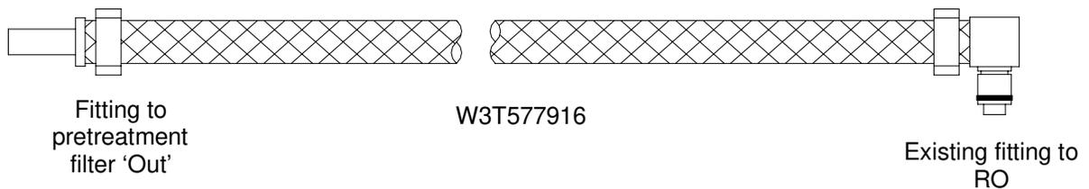
2. Measure approximately 6" from the pretreatment filter fitting end of hose. Cut hose. Keep the 6" length of hose with the pretreatment fitting end. Discard the remaining length of hose with the existing QD (quick disconnect).
