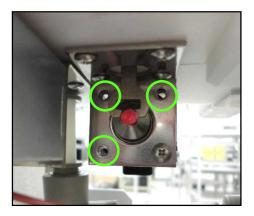
5. While holding the solenoid from the backside, remove the final screw. After the screw is removed, tilt the solenoid to free it from the rocker arm and pull the entire assembly out from the bracket. Plunger may fall out, take care not to lose plunger and spring.
