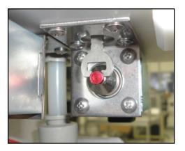
11. Re-insert the electrical connection to solenoid.
