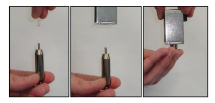
8. Place a screw on the screwdriver to be ready for re-installation in the next step. NOTE: The screw is non-magnetic and may fall off worn screwdrivers.
