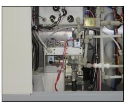
3. Remove the electrical connection to the SV4 Solenoid (SV4 is the solenoid with the red mark on the end of the plunger).
