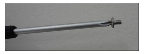
9. Keeping the solenoid tilted plunger side up; insert the solenoid back through the bracket and install one of the bottom screws (do not fully tighten).
