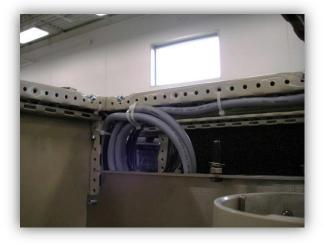
9. Disconnect the water saver line from the lower manifold.
