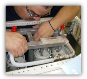
24. Place nylon spacers (P/N W2T915041) on threaded studs of upper bracket supports. Reinstall upper angle brackets, set in place.
