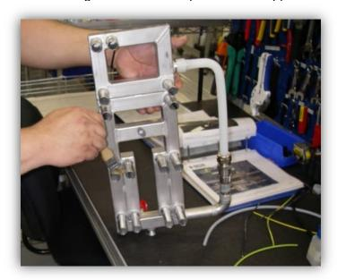
23. Reinstall upper manifold. Use care not to damage O-rings.
