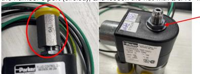
Once the nut is loosened, the valve end will be able to be rotated. Orient the number 2 port away from the power cord end and the number 1 port on the power cord end. Tighten the nut once the valve end is properly oriented. Do not overtighten. Tape the threads on one elbow, one tee, and one connector. Install the elbow in the number 2 port. Install the connector in the number 1 port. Reinstall port number 3. Install the tee in the number 3 port. The proper orientation is shown below.
