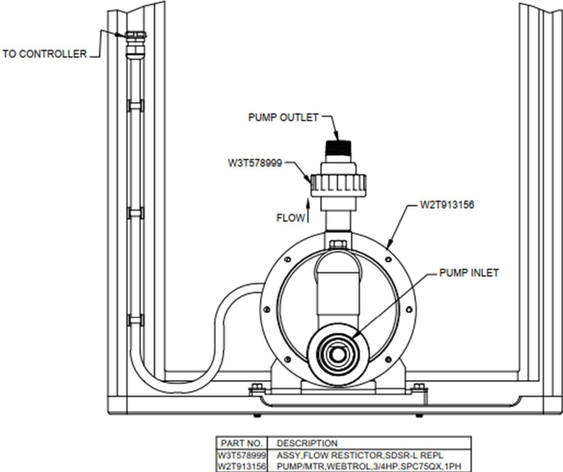
Illustration 6.23: SDS Mix Pump Replacement Parts
