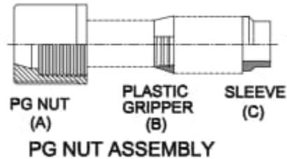
AS SHOWN ABOVE, INSERT GRIPPER (B) INTO NUT (A).
