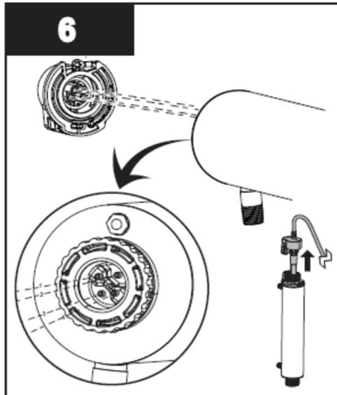
7. Push the lamp connector against lamp connector base together until an audible click is heard. Restore power and re-pressurize the system to check for leaks.
