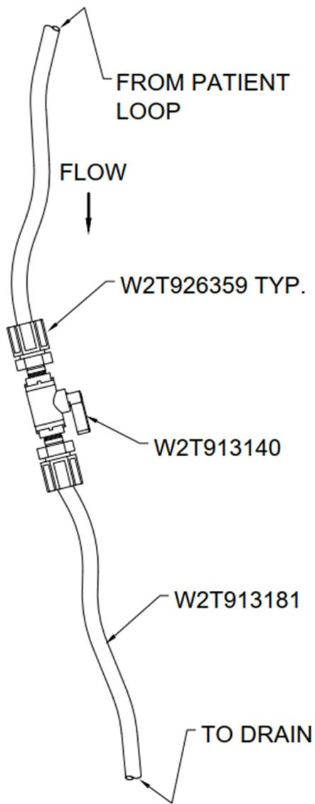
Figure 2.8: Acid Loop Return Assembly
