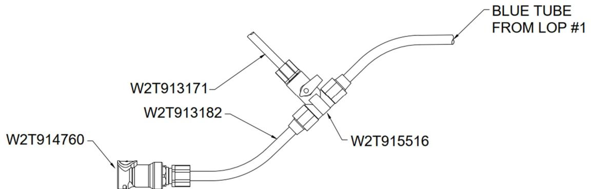
Figure 2.5: Single Loop Bicarb Wand
