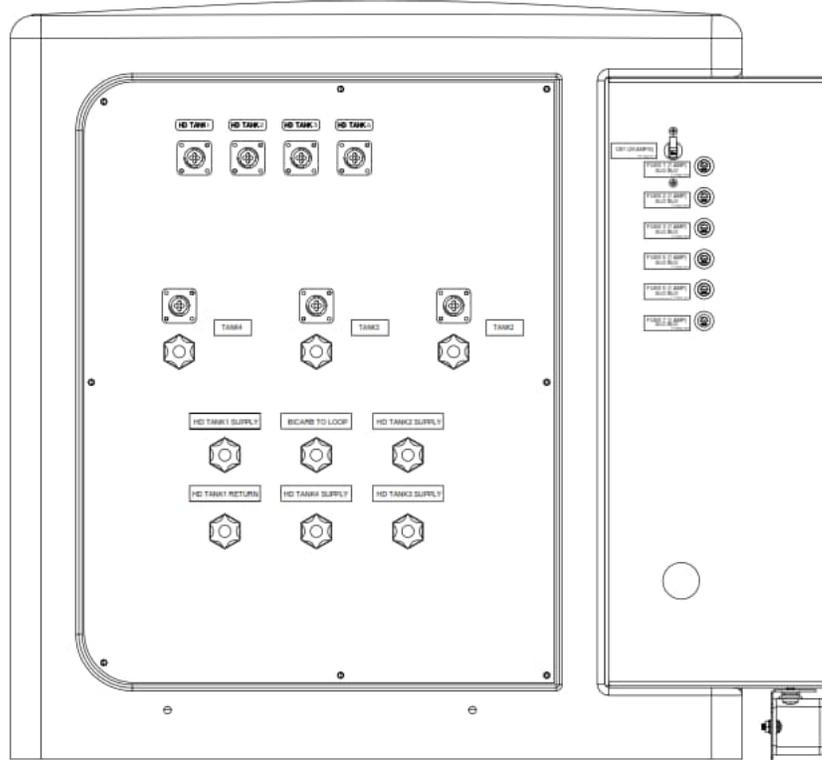
Figure 2.4: SDS Mix Frame Tube Connections (Three Acid)
