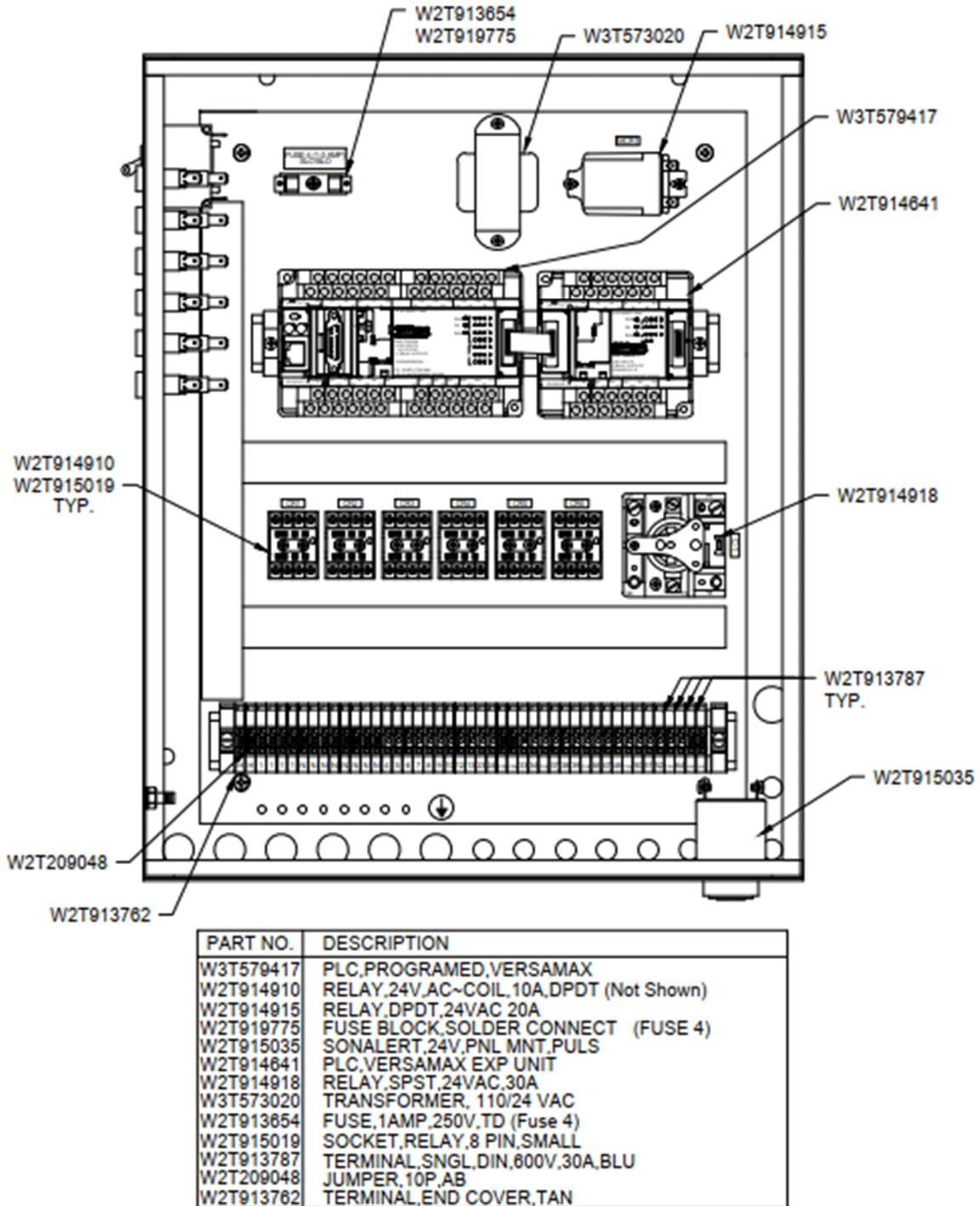
Illustration 6.6: SDS Electrical Controller Components
