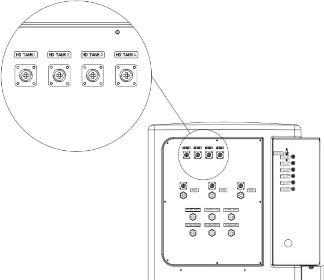
Illustration 6.16: SDS Head Tank Wiring Connections
