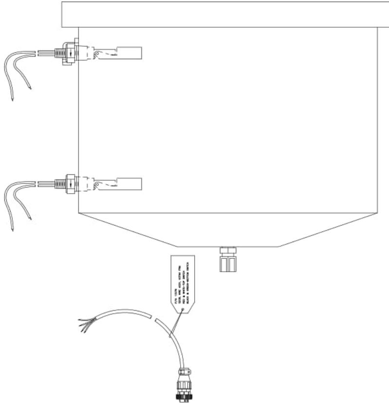
Figure 2.3: Head Tank Electrical Connections
