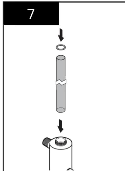
8. Reinstall the top and bottom retaining nuts, floating spring, and O-rings respectively. When service is complete, assemble the prerequisites in the reverse order of disassembly.
