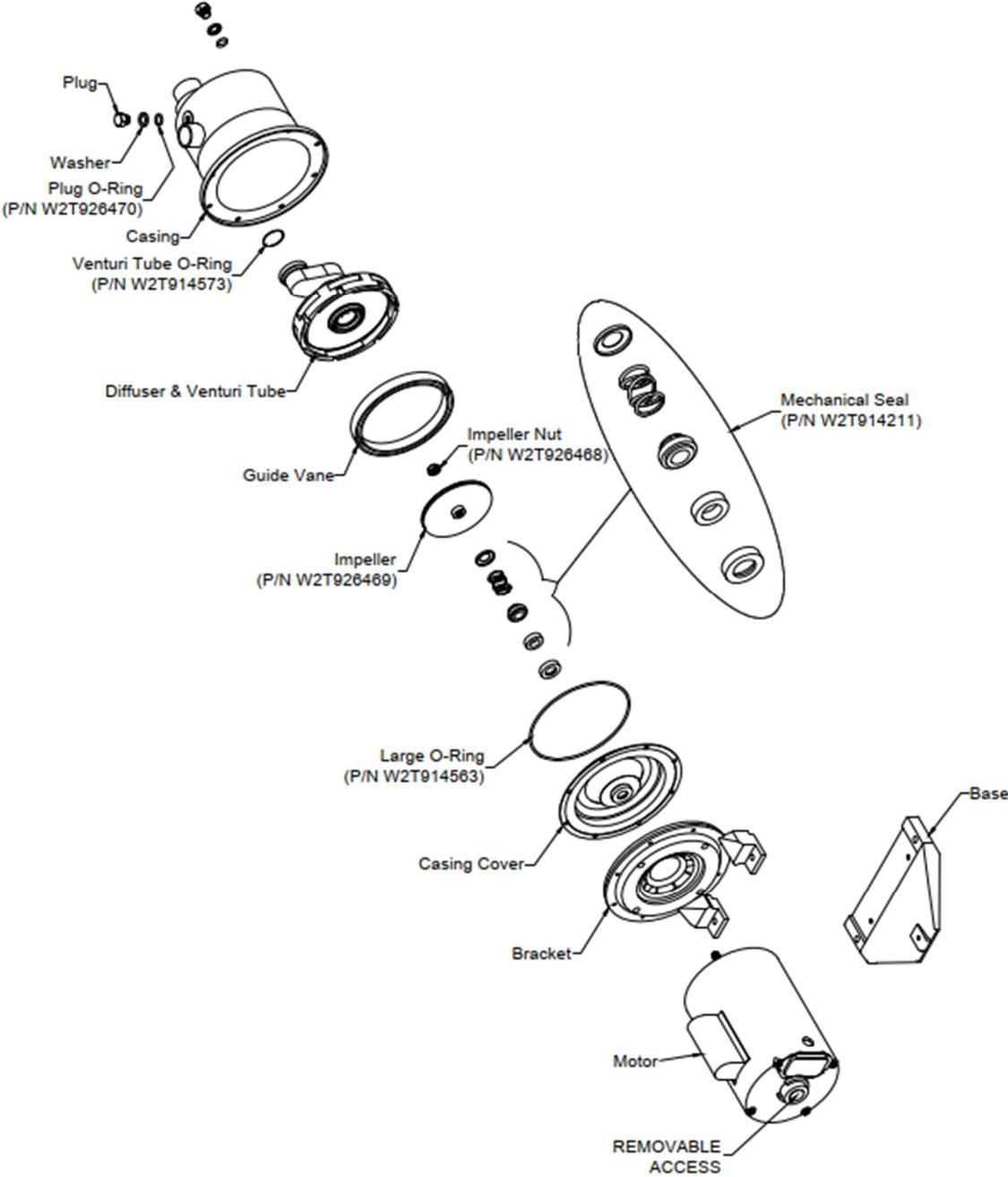
Illustration 6.24: SDS Pump/Motor Detail
