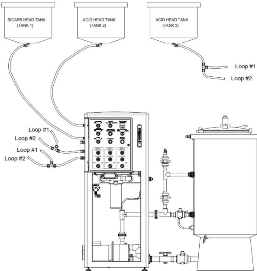
Figure 2.2: SDS Head Tank Tubing Installation
