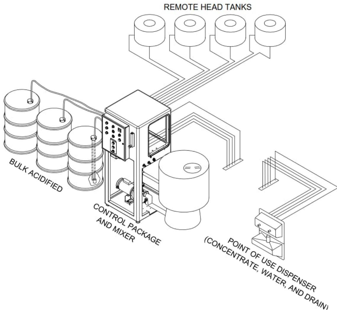
Figure 2.1: SDS System Diagram
