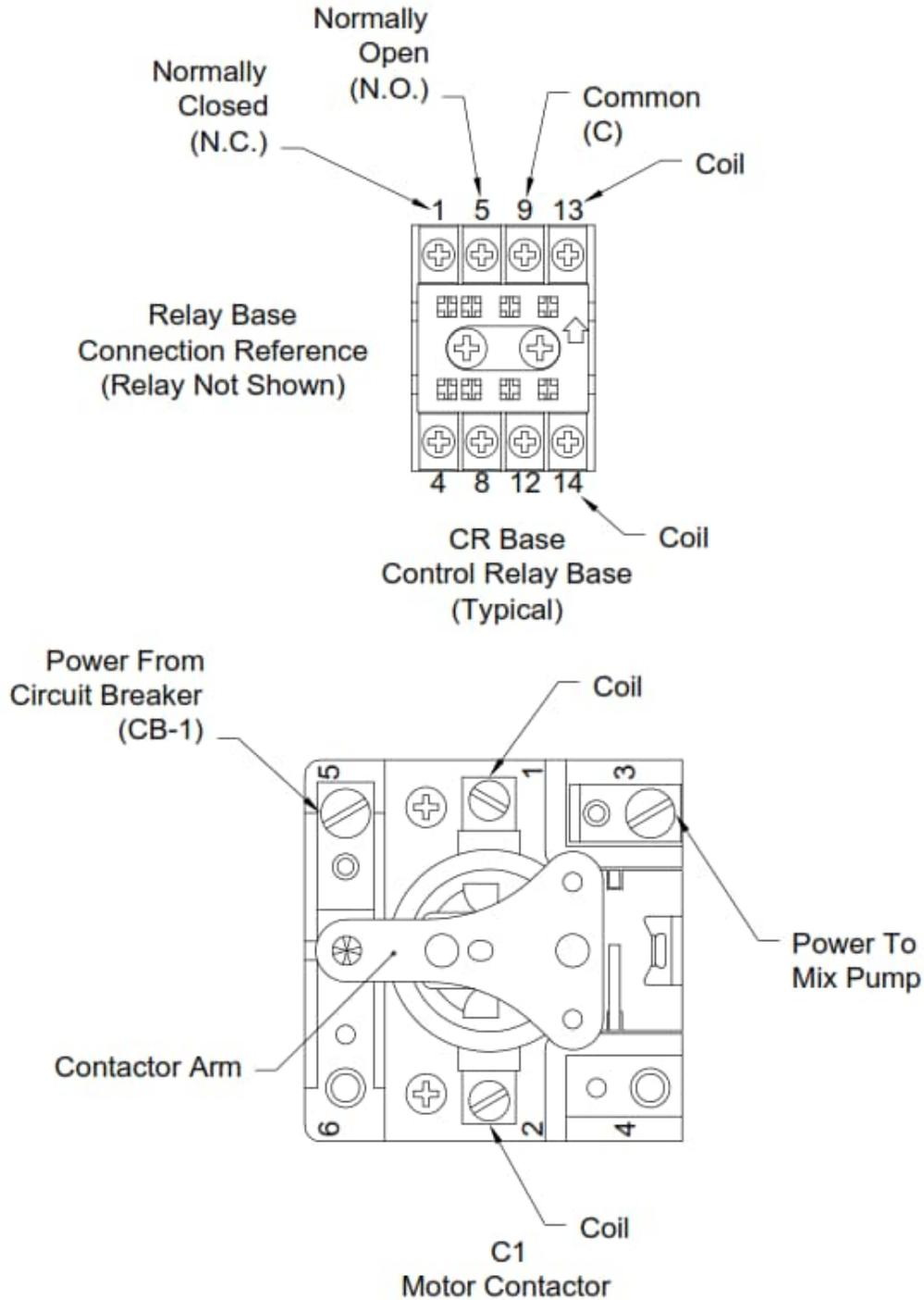
Illustration 6.8: Electrical Components (Control Relay and Motor Contactor)
