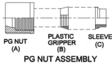
AS SHOWN ABOVE, INSERT GRIPPER (B) INTO NUT (A).
