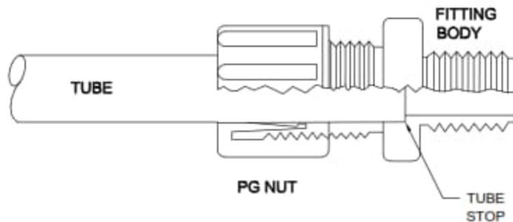
NOTE: IT IS NOT NECESSARY TO DISASSEMBLE THIS FITTING FOR APPLICATION. MERELY INSERT TUBING TO STOP AND TIGHTEN NUT.
