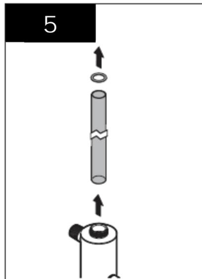
6. Clean the quartz sleeve with a cloth soaked with vinegar or some other mild acid and then rinse with water. The exterior and interior surface of the quartz sleeve should be cleaned. Running either a cotton swab or non-abrasive brush through the interior of the quartz sleeve can do this.
