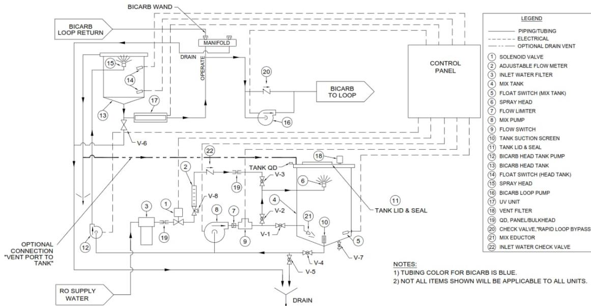
Figure 3.2: SDS Bicarb Process Diagram
