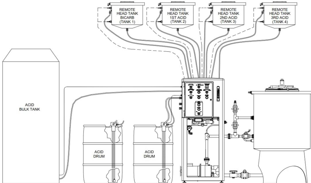
Figure 2.9: SDS Remote System
