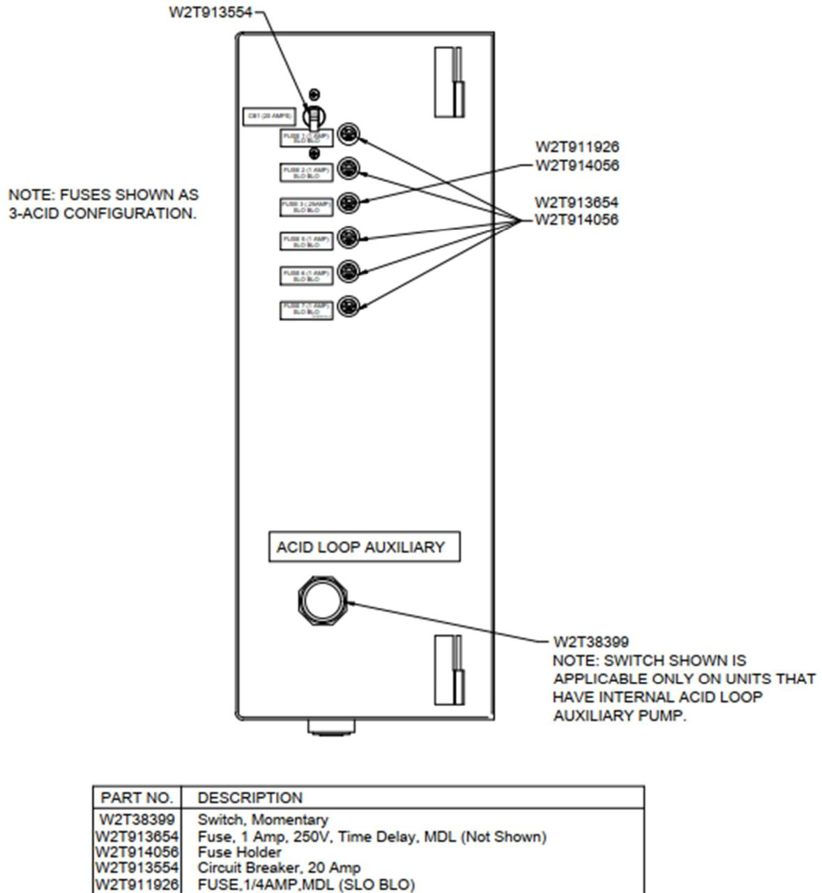
Illustration 6.10: SDS Controller (Left Side View)
