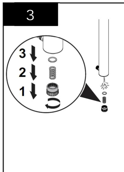
4. At the connector end, remove the retaining nut (1) and O-ring (2).
