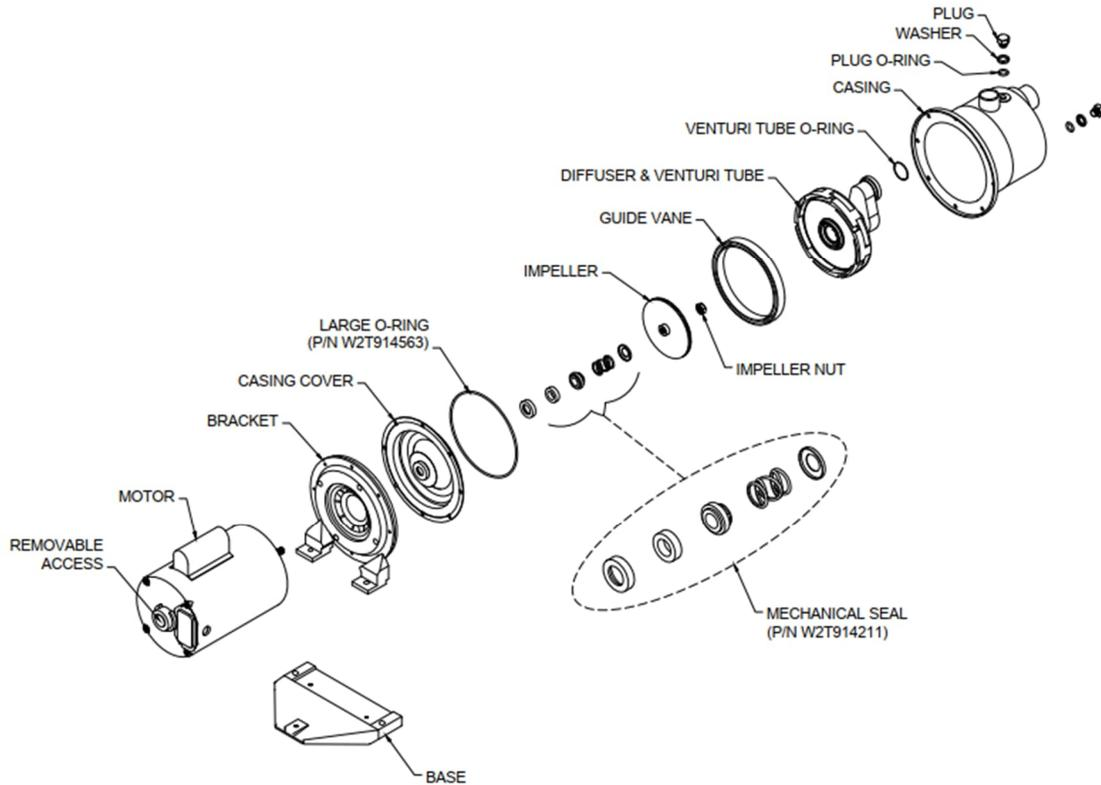
Figure 4.2: EBARA Pump Exploded View
