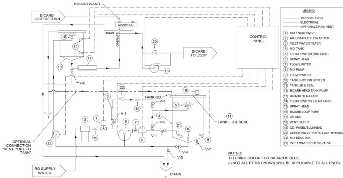
Figure 3.3: SDS Bicarb Process Diagram
