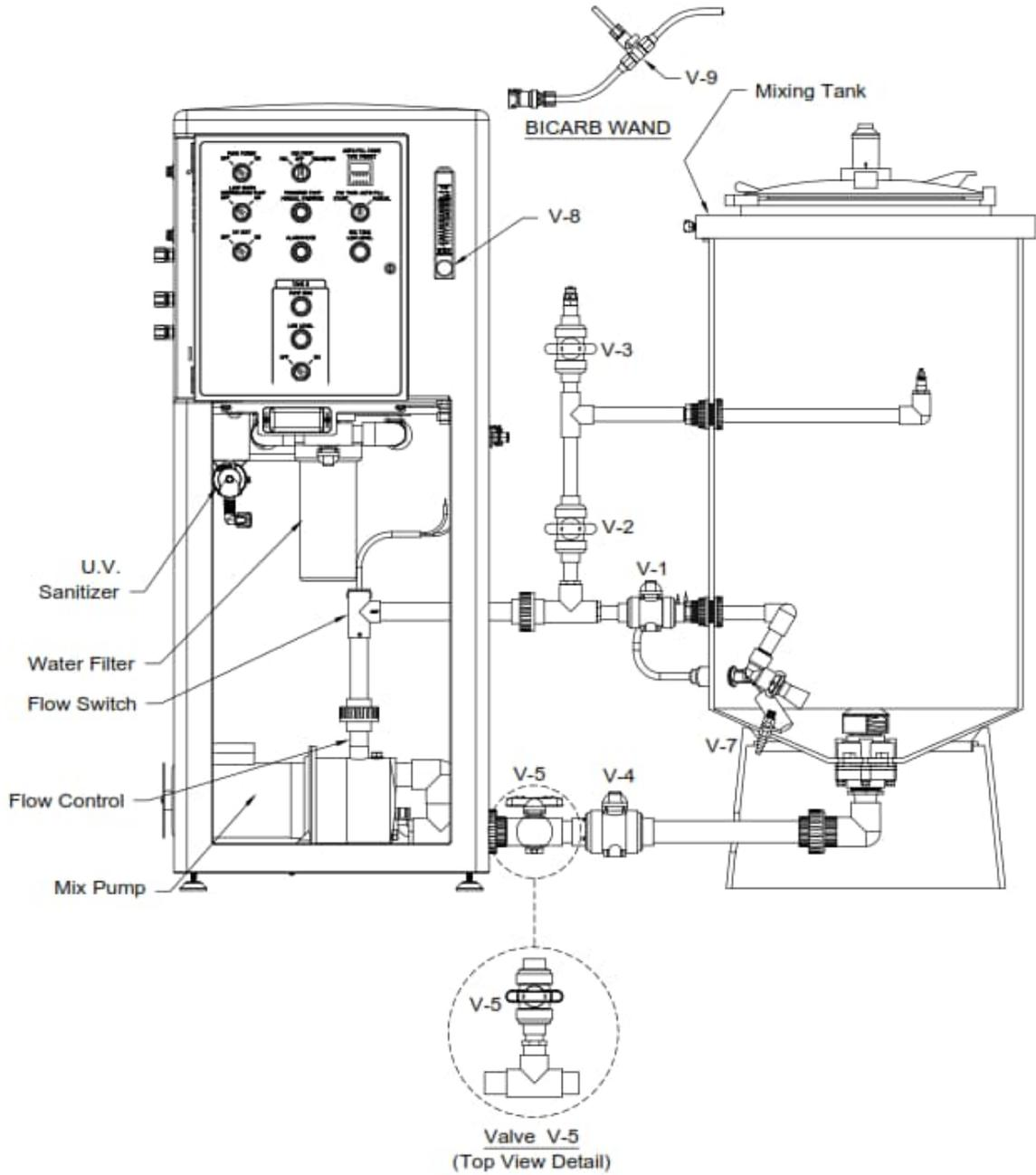
Illustration 6.1: SDS Frame and Mix Tank with Valve Callouts
