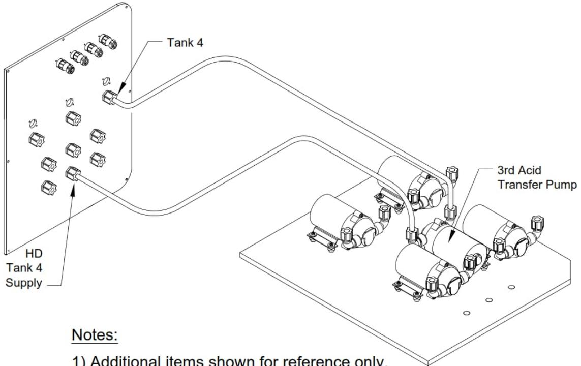
**Illustration 6.21: SDS 3rd Acid Head Tank Pump Tubing
