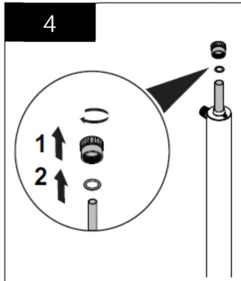
5. Carefully, remove O-ring adhering to the quartz sleeve. Remove the quartz sleeve.
