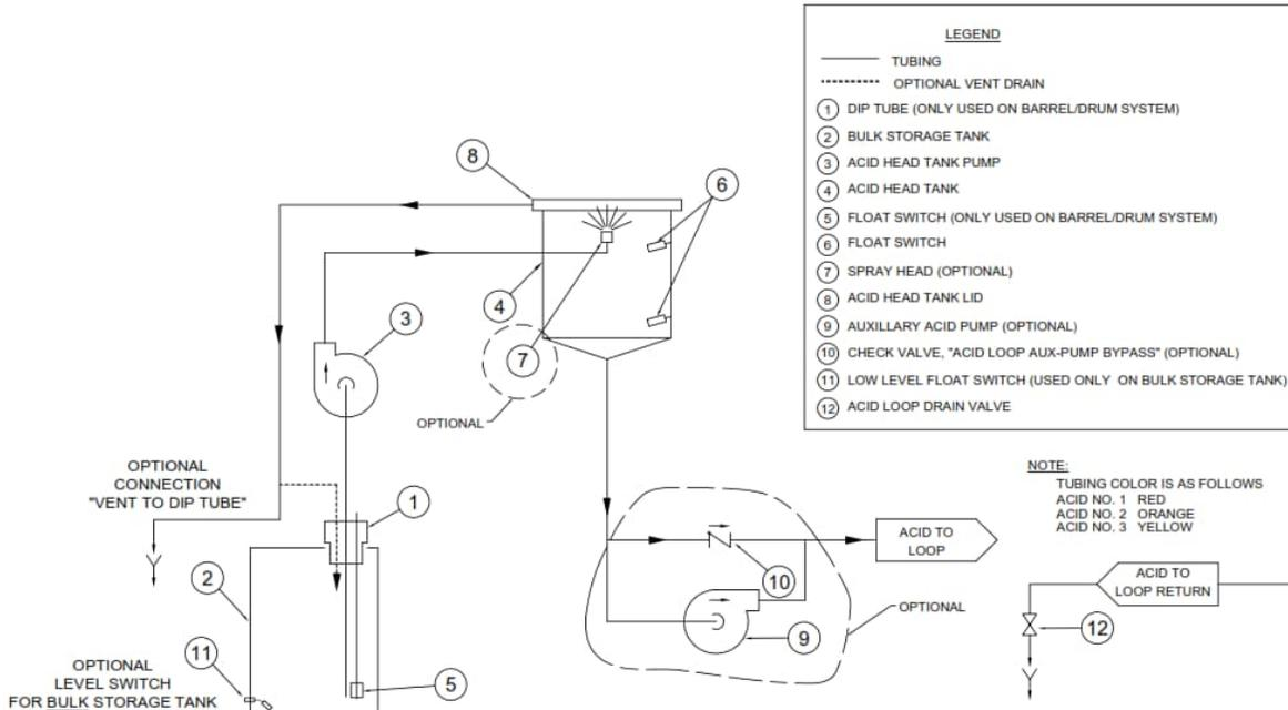
**Figure 3.1: SDS Acid Process Diagram**
