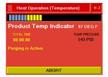
21. Once the purge process is complete, the RO's internal water is circulated and heated to a target temperature of 176°F (80°C).
