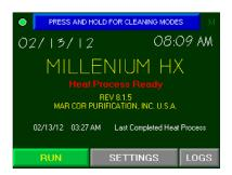
9. Verify the time and date on the RO. If they need to be adjusted, touch in the area of the time and date and follow the on screen instructions to adjust. The time does not automatically adjust for day light savings.
