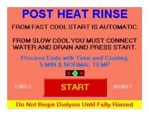
13. Connect the RO to water and drain (if not already connected) and press START to begin the post heat rinse.
