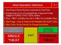
20. The machine starts to purge, filling the internal tank to the proper level with product quality water.
