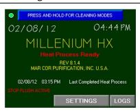
17. Press and hold the blue banner at the top of the screen that states PRESS AND HOLD FOR CLEANING MODES to enter the Chemical or Heating Operations selection screen.
