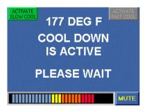
24. After the RO reaches 120°F (49°C), the RO will enter a POST HEAT RINSE. This will further cool and rinse the RO for a minimum of 5 additional minutes.
