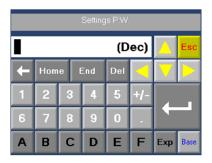
29. Press the PRODUCT QUALITY ALARM. Once in the set point screen, set the alarm set point per facility protocol or if no protocol exists, set at two times the steady state operating TDS ( $\mu$ S). Once complete, press  $\blacksquare$ .
