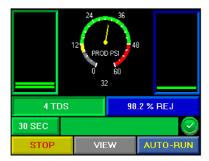
8. Let RO run for 15 minutes from when the start button was pressed to ensure pre-RO devices are flushed. Test pre-RO devices to ensure they are operating within specifications.
