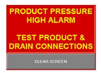
This function is active during all operations of the Millenium HX and if triggered will stop the pump and sound an alarm. This set point is set in the code at 60 PSI.
