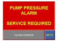
This alarm is active at all times as a high and low pressure watch. If this alarm is triggered, the pump will shut down. The levels at which the alarm will activate are based on the mode, water temperature, and pump pressure set points. The alarm set points can not be changed.
