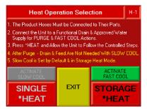
5. The machine starts to purge filling the internal tank to the proper level with product quality water.
