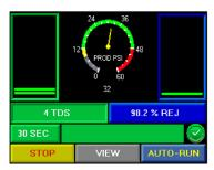
2. When AUTO-RUN is pressed, the operator can set the RO to run for up to 59 minutes at specified time intervals (1 minute up to 99 hours and 59 minutes). To enter time, press the box indicating the time. When the RO is running, the IDLE indicator is replaced with OPERATING. To exit, press the CANCEL & EXIT banner. When pressed, the RO will exit back into the normal run screen starting in a startup flush with product water diverted to drain.
