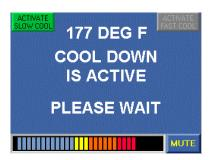
9. After the system cools to a temperature of 120°F (49°C), the screen moves to a POST HEAT RINSE screen. If the RO is in Fast Cool and water and drain are supplied, the machine will automatically start in POST HEAT RINSE. If the RO is in Slow Cool, the operator must connect the RO feed water and drain and press START to begin the post heat rinse.
