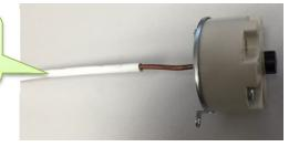
Check if the High Limit Switch has "tripped"; the blue reset button would be extending 1.7 mm past the black "set plug". The High Limit Switch should not "trip" during normal heat disinfection if it is within tolerance. Reset the High Limit Switch if it has tripped. If the problem persists order a replacement switch, 3028896.
