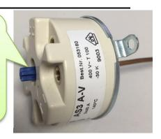
Confirm a white insulating sleeve is not present on the copper probe of the High Limit Switch. If one is present, remove and discard as it is not necessarily and may retain heat, refer to the figure below.
