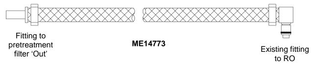
2. Measure approximately 6" from the pretreatment filter fitting end of hose. Cut hose. Keep the 6" length of hose with the pretreatment fitting end. Discard the remaining length of hose with the existing QD (quick disconnect).
