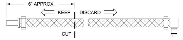
3. Install straight male QD from WRO 300 install kit WT300INSTKIT01 using hose clamp from same kit.
